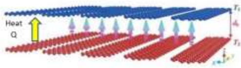
Figure 5. Near-field heat transfer - Graphene Ribbons
